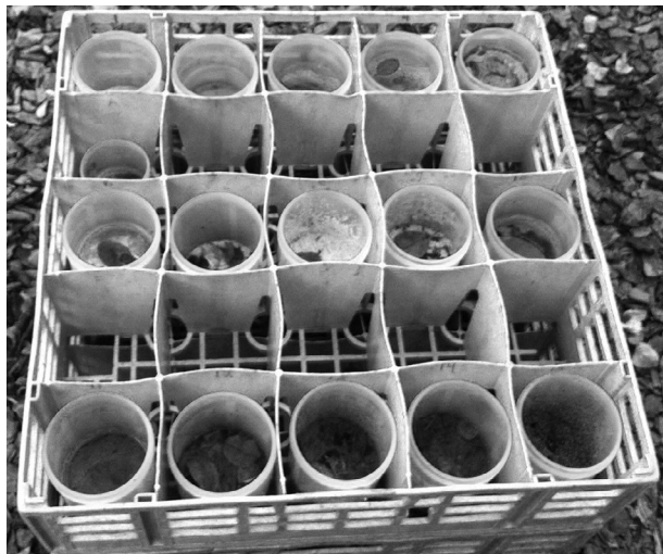
Fig. 3. Samples in the restricted-access courtyard (41.29°N, 82.22°W, 247 m). The top row, from left to right, is: kaolinite, illite, muscovite, vermiculite, and montmorillonite. The middle row, from left to right, is quartz sand <63, 63–125, 125–250, 250–500, and 500–850 \mu\text{m} . The bottom row, from left to right, is river sand <63, 63–125, 125–250, 250–500, and 500–850 \mu\text{m} . The single container on the far left between the top and middle rows is the rainfall beaker where we collected rainfall during each period. A rain gauge is to the left of the apparatus (outside of the photo) next to the middle row of containers.
